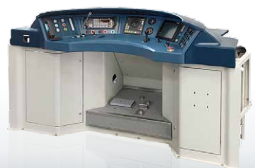
Pre-assembled component: Driver desk
